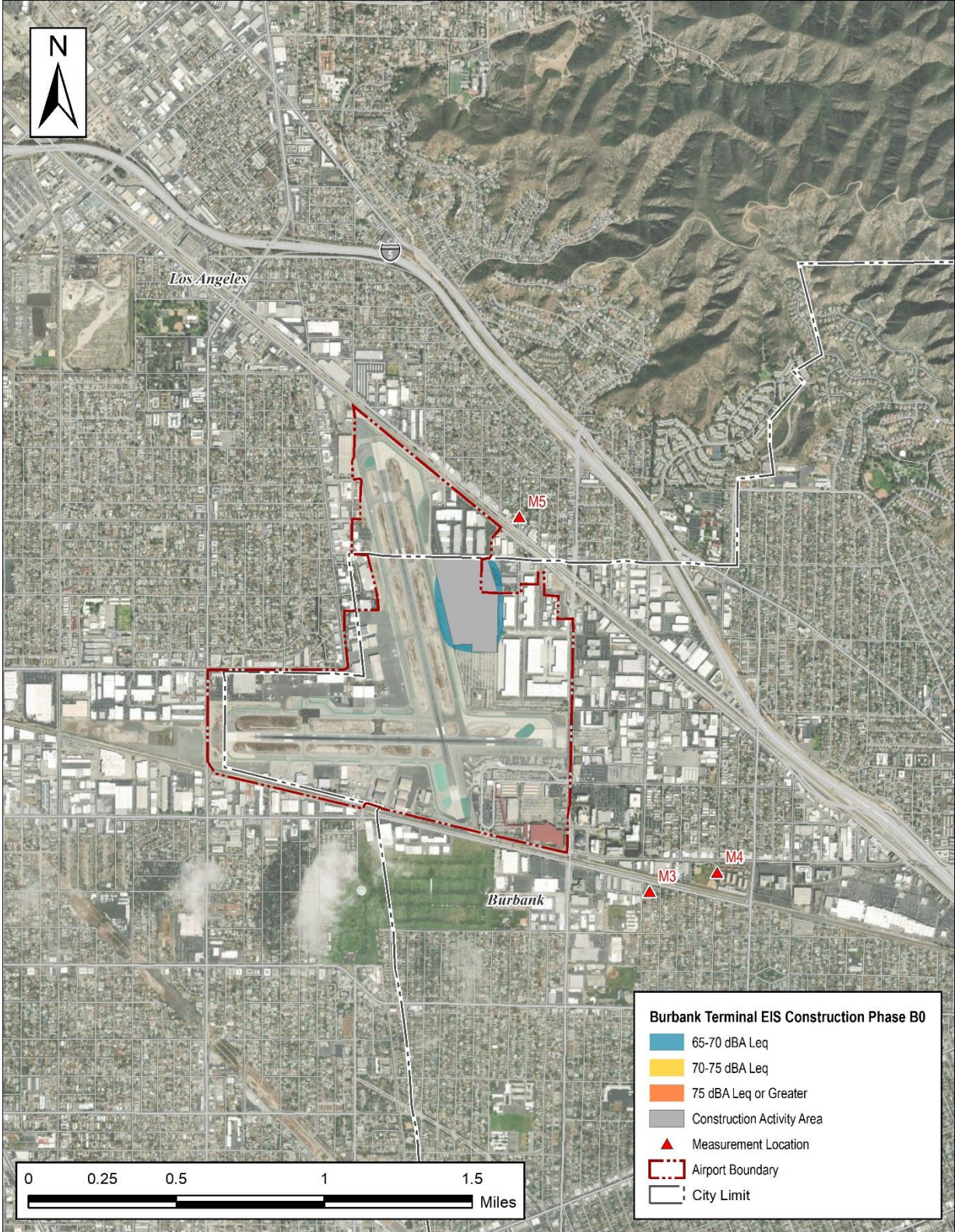
Figure 6. Construction Phase B0 dBA Leq Noise Contours
