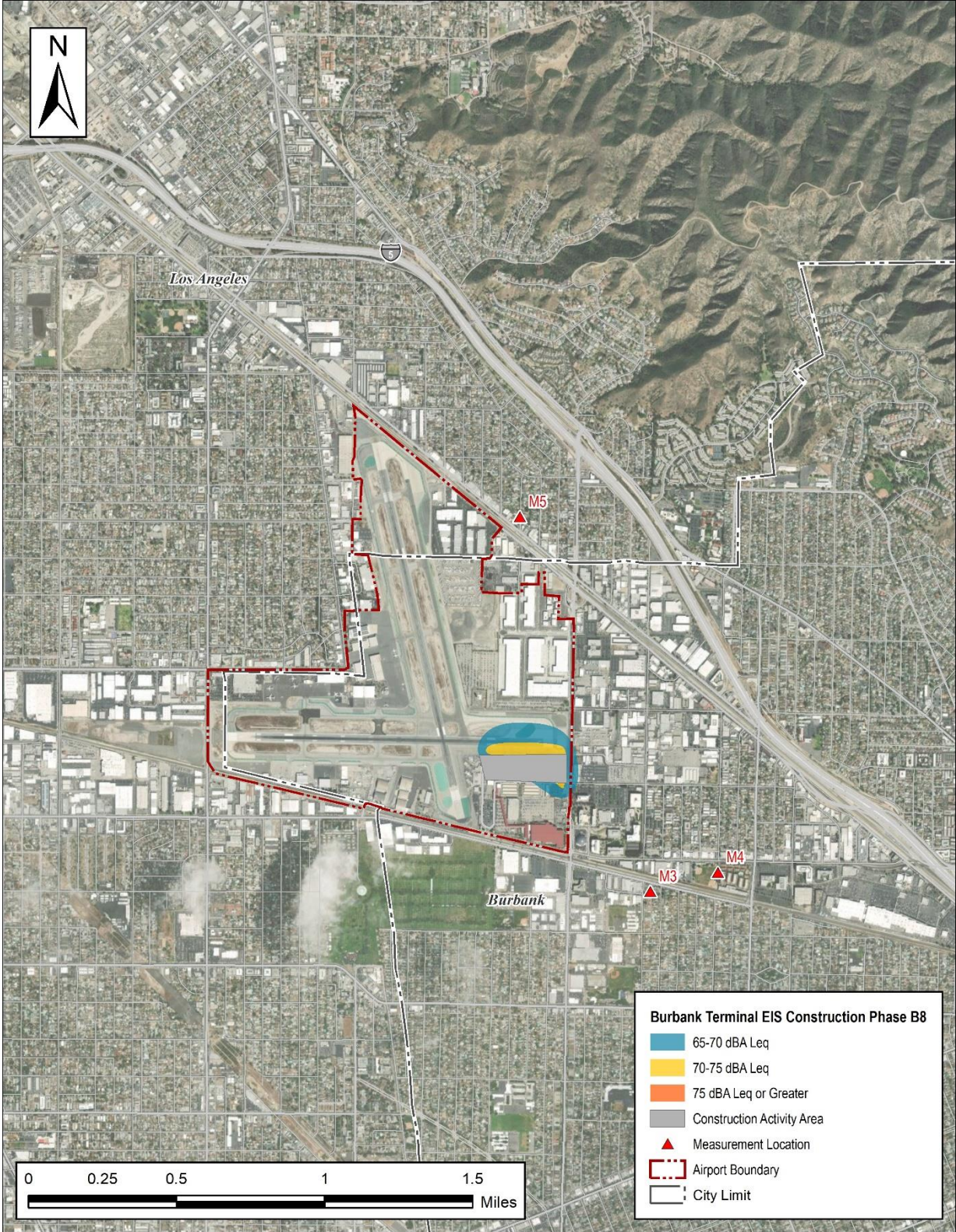
Figure 15. Demolition Phase B8 dB Leq Noise Contours
